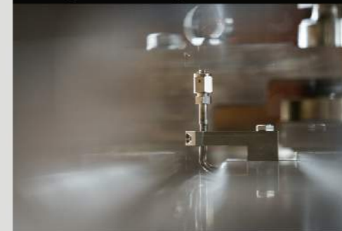
VCR connection for permanent bellows leakage monitoring
