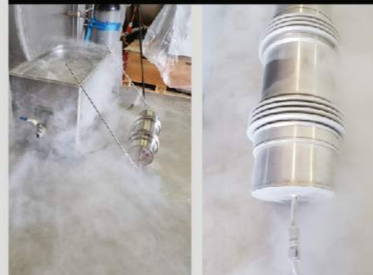
Cryogenic shock test before leakage test
